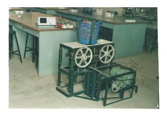
Figure 2 Set up with the fresh tomato fruits packaged in the plastic basket (PM2)
