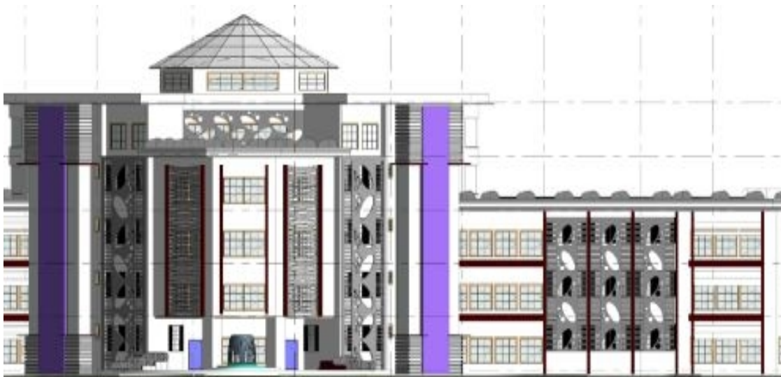
Figure 4.6: Atrium, windows and vents in the proposed design (Source: Author, 2019)
