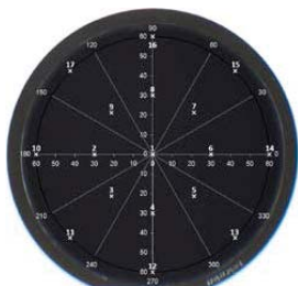
Figure 1 : Map of measurement points superimposed on 6 inches anodized wafer.
