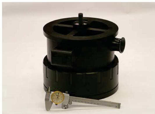
Figure 1. Assembled anodisation cell prototype made of HDPE
