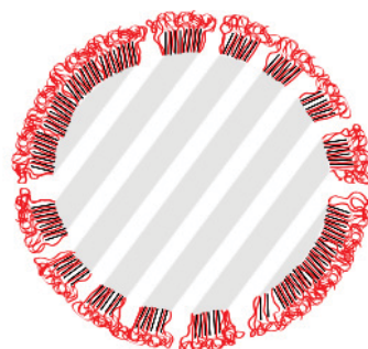
Figure 1. Dual PEGylated TOPSi NP showing two conformations of the PEG layers: 0.5 kDa PEG forming brush-like layer (black) and 2 kDa PEG forming mushroom-like layer (red) at the top of 0.5 kDa layer.
