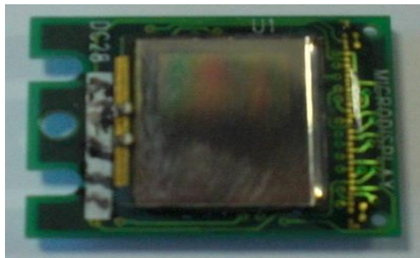
Figure 2. Structure and external view of microdisplay
