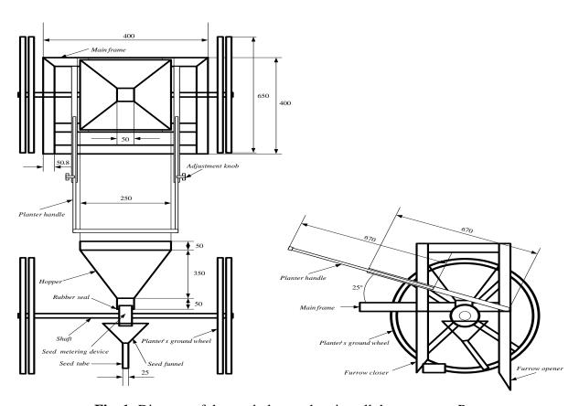
Fig. 1: Diagram of the seed planter showing all the necessary Parts
