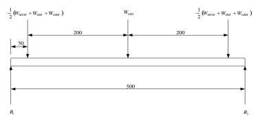
Fig.2: Load distribution on shaft
