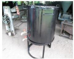
Plate 1. Constructed Local Improved rice Parboiler
