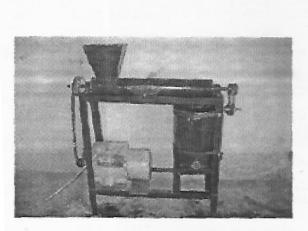
Fig 5: The Constructed Locust Bean Dehuller and Separator
