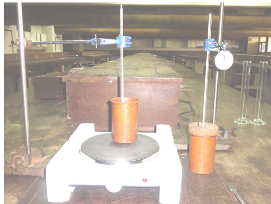
Figure 4. Set up for determination of thermal diffusivity of melon seeds
