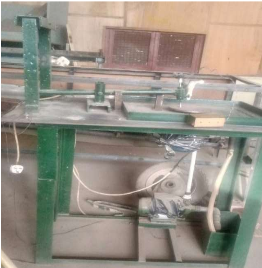
Figure 4.1: Dual Condition Pin-On-Disc Wear Testing Machine
