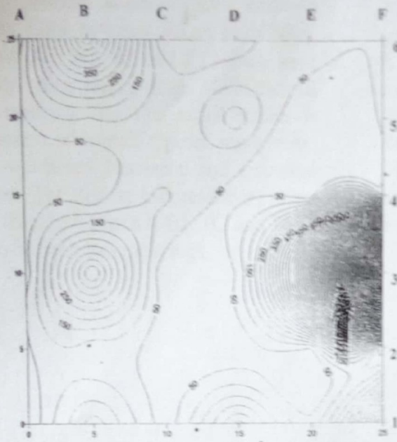
Distance (m) x 10 on both axes Figure 10: Iso-resistivity contour map at 5m Contour Interval 50 ohm-m
