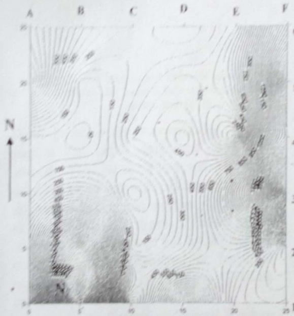
Distance (m) x 10 on both axes Figure 14: Iso-resistivity contour map at 25m Contour Interval 50 ohm-m
