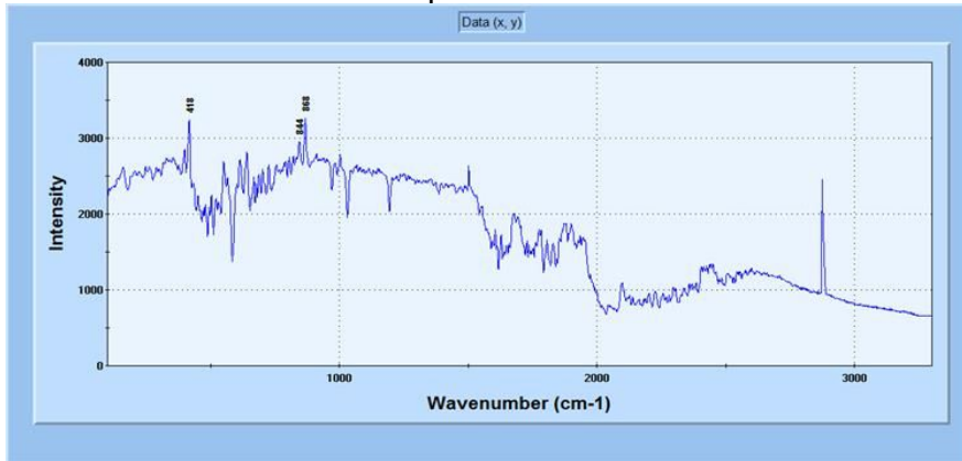
Figure 4: FTIR for Quartzite ore powder
