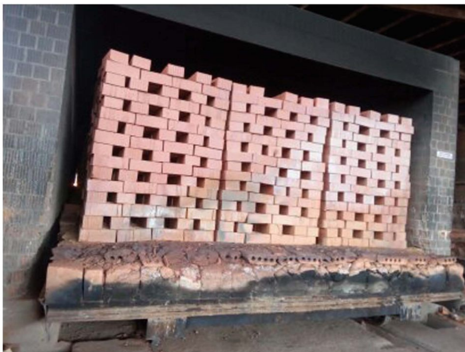
Fig. 3. Clay bricks after firing from the furnace
