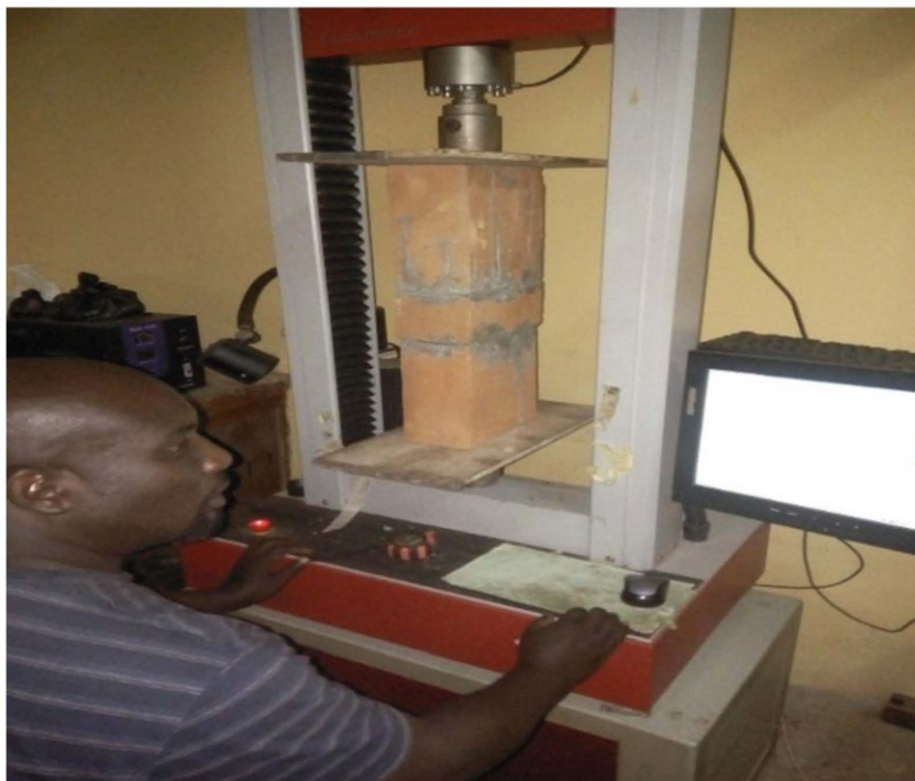
Fig. 5. Compressive test on clay brick
