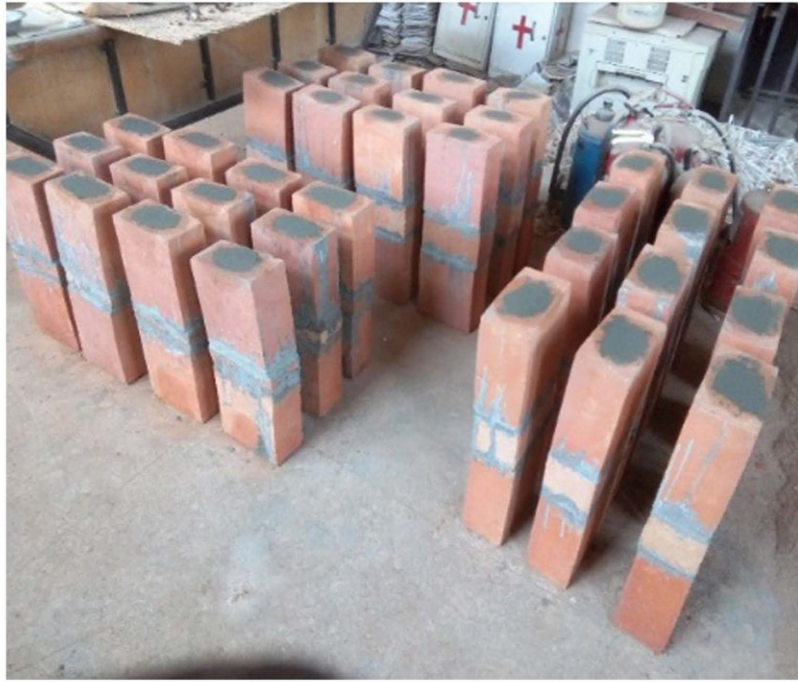
Fig. 4. Interlocked clay bricks
