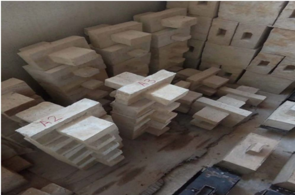
Fig. 2. Freshly demolded clay brick components
