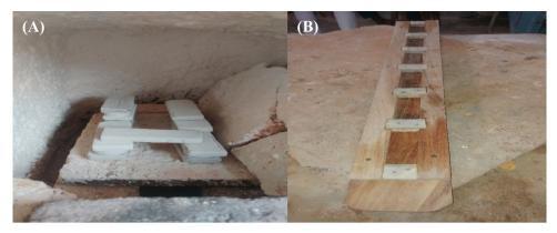
Plate 1. (A) Trial bars prepared from beneficiated kaolin and (B) Mould.
