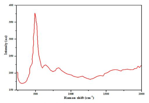
Fig. 3. Analysis of kaolin using Raman spectroscopy.
