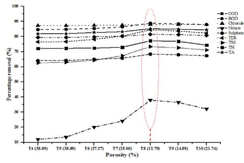
Fig. 8. The total removal efficiencies of the second scrubbed pot filters.
