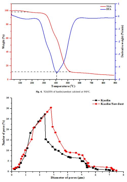
Fig. 5. Pore size distribution of kaolin and kaolin/sawdust sinter at 910 °C.
