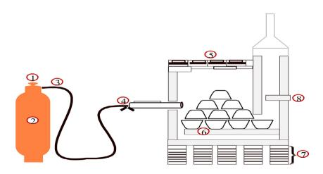
1. Tap 2. Gas cylinder 3. Nozzle 4. Burner 5. Roof parts 6. Internal floor 7. Pillars 8. Chimney
