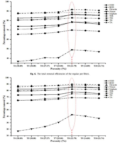
Fig. 7. The total removal efficiencies of the first scrubbed pot filters.
