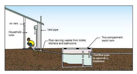
Figure 5: Septic tank system (Reed, 2014)
