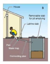
Figure 4: Direct (A) and offset (B) Pour-flush latrine (Reed, 2014)
