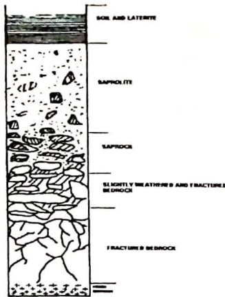
FIG 5: Subsurface cross section in hard rock terrain (Idowu and Ajayi, 1998)
