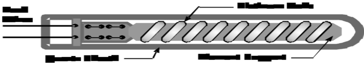
Fig.1.3: Diagram showing a structural view of a resistance thermometer transducers
