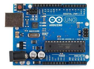
Fig. 3 Arduino Microcontroller board [8]
