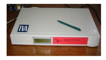
Fig. 1. Frequency disturbance recorder (FDR)
