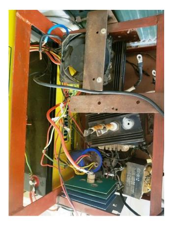
Fig 9: Photo view of the 220V A.C to 24V D.C Circuit
