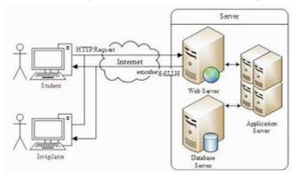
Figure 3. EEV System Architecture
