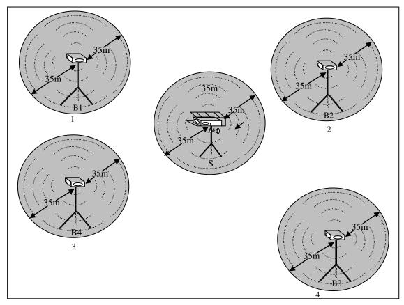
Figure 2: Isolated Placement Method of Ultrasound Boosting in a Hypothetical Farm
