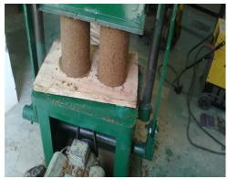
Plate 7. Ejection of briquettes from machine.
