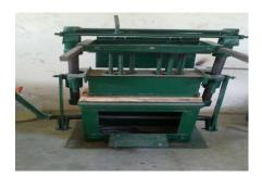
**Plate 1.** Motorized vibratory briquette making machine.
