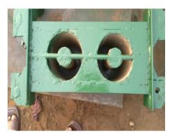
Plate 3. Machine mould unit.
