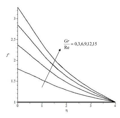
Fig. 2. Velocity profile for different values of Gr/Re,  $\lambda$ =0.3,M=1.0, $\Lambda$  = 1.0,Ec=0.1, Ha=0.1 and Da=0.1
