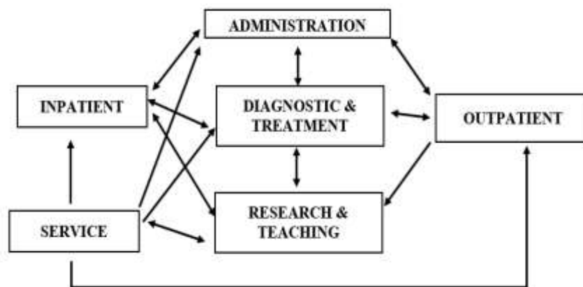
Figure 1: Flow Diagram of Various Units in a Modern Healthcare Facility. (Source: Thomas, 2006).
