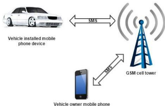
Fig.1. Physical architecture of the theft alert function
