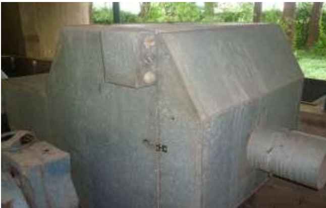
Fig. 10: Platform Sugar Dryer
