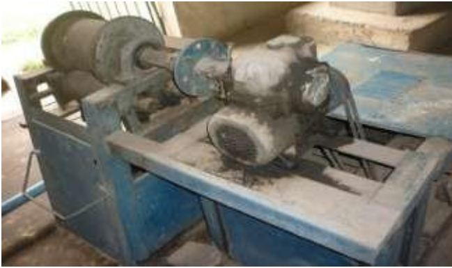
Fig. 3: Roller Juice Extractor
