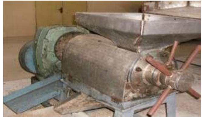
Fig. 5: Cane Juice Expeller
