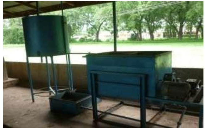
Fig. 8: Combined Air/Water Cool Crystallizer System
