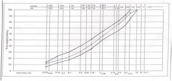
Figure 1b: Obtained From the Combined Gradation of Artificial Aggregate.
