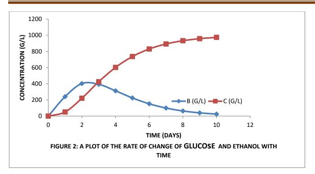
The plot of glucose yield and ethanol production is given in Figure 2. As the glucose yield increases the ethanol also increases until after day 2 when it starts decreasing due to the utilization of the available glucose for the ethanol production.
