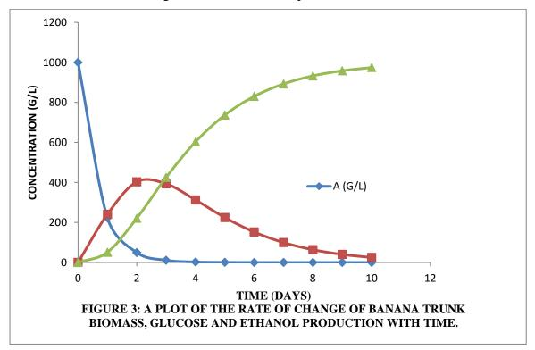
The graph for the kinetics of ethanol produced from banana trunk biomass is given in figure 3. The rate of change of ethanol with time is inversely proportional to that of biomass.
