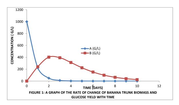
Figure 1 shows the dynamics of banana trunk biomass and glucose yield. The banana trunk biomass decreases at the rate of  $\alpha = 1.5$  from the initial value of 1000g/l to 0.000305902 g/l at day 10. The glucose yield increases from day one at the rate of 0.8 to an optimum yield of 403.172636g/l at day two.
