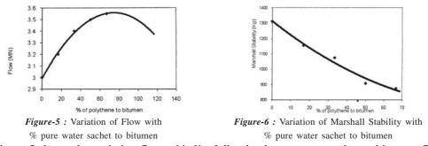
Figure 5 shows the variation flow with % of dissolved pure water sachet to bitumen. This indicates that the more the replacement of bitumen with dissolved pure water sachet in the asphalt mixes the more its potentials to deformation which has implication on the sliding of pavement when it is subjected to use by traffic.
