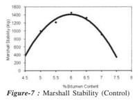
350kg for Nigeria roads. This implies that the capability of the resulting Asphalt mix can withstand heavy traffic loading of Category E and F which is equivalent to about 4,500vpd exceeding 30tons loaded weight. (5).
