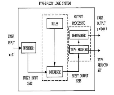
Fig. 1. 1. The structure of a Type-2 FLS (Mendel, 2003).
