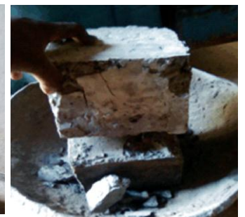
Plate 2: Crushing Test Plate 3: Failed PKS concrete cube
