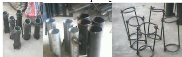
Plate 1: materials used for strengthening the openings
