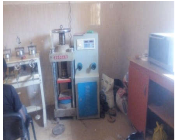
Plate 2: Flexural strength testing machine of 2000kN capacity
