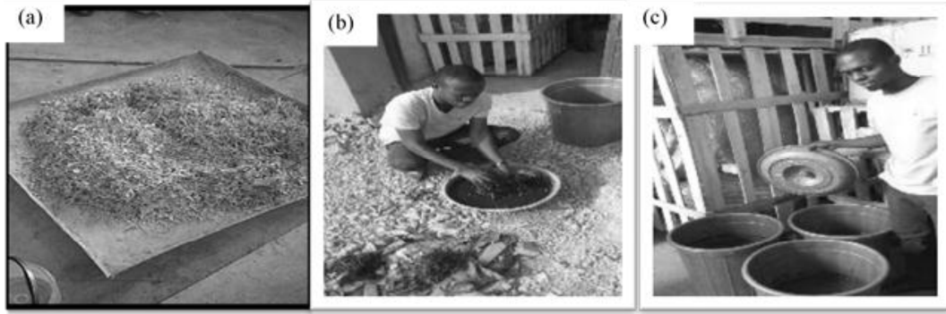
Figure 2. (a) Locust Beans Pod after grinding into fibers, (b) Sieving of extract, (c) Extract inside basin
