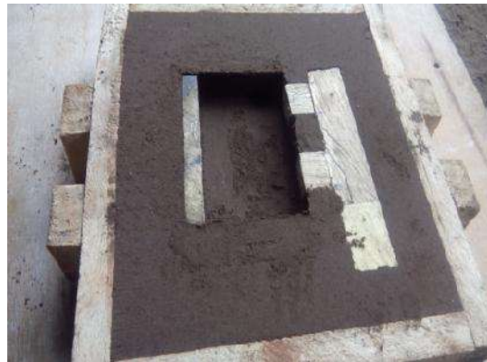
Figure 2: Brass Chill and Gating in position
