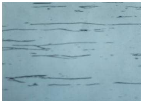
Plate 1: Microstructure of (as-received) of ASS 304L (Etched) using a solution of 10ml HNO 3 + 30ml HCL and 10ml glycerol for 2mins.
