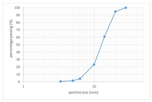
Fig. 2: Sieve Analysis for crushed coconut shell
