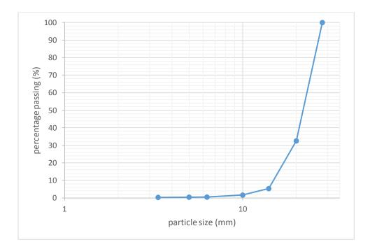
Fig. 3: Sieve Analysis for gravel (crushed aggregate)
