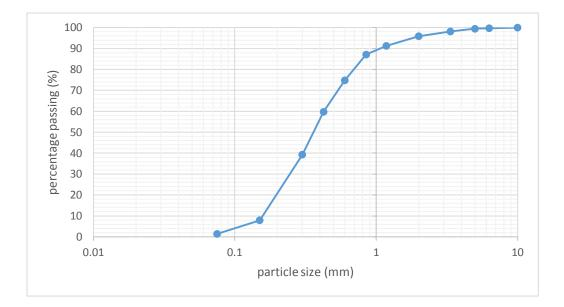
Fig. 1: Sieve Analysis for Fine Aggregate
