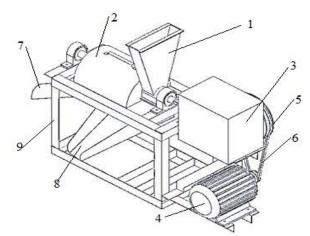
Figure i. Diagram of the fish oil extruding machine
