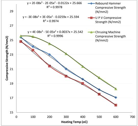
Figure 1: Compressive Strength against Heating Temperature
