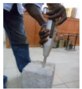
Plate I: Testing Using Schmidt Rebound Hammer
