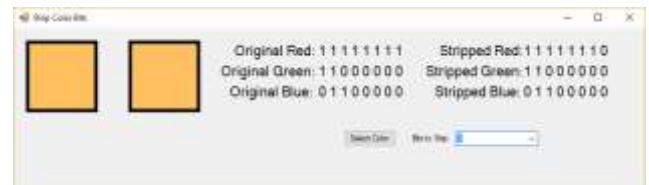
Figure 6: This color can be seen in its original hue in the rectangle to the left. With a single bit shaved, the new color can be seen in the second rectangle. There is no perceptible difference between the original color and the color that has had the least significant bit shaved.
