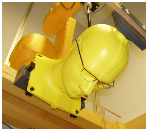
Fig 1 SAR measurement setup showing 900MHz dipole in horizontal alignment and a pair of semi-rimmed spectacles mounted on the SAM head
