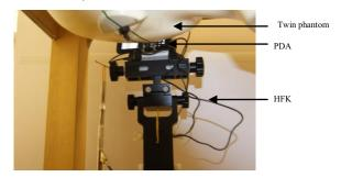
Figure 7: Picture of wire position for third HFK wire scenario.
