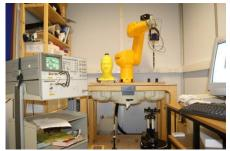
Figure1: Experimental setup for SAR measurement.
