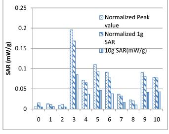
Figure 6: The SAR values in the ear when the HFK wire was placed in random positions (1-10) and smart phone without HFK.
