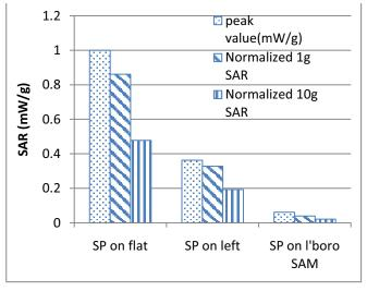
Figure 5: Graph of the smart phone (SP) in different positions on the phantoms without the HFK.
