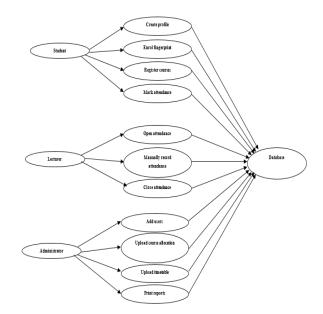
Fig. 2. Functional Diagram of Wireless Fingerprint-based Attendance System
