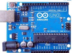
Fig. 2: Arduino UNO R3 Board (Tutorialspoint, 2018)
