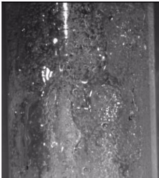
Figure 6: Video image of slug flow for a riser at liquid superficial velocity = 0.142 m/ s and gas superficial velocity = 0.544 m/ s.
