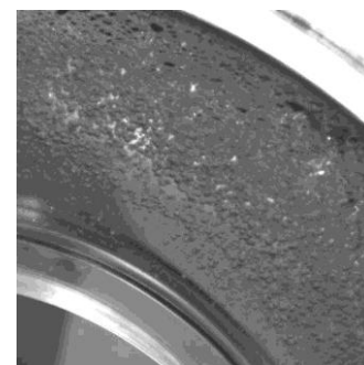
Figure 9: Video image of spherical cap bubble flow passing through a vertical 90 degree bend at liquid superficial velocity = 0.142 m/ s and gas superficial velocity = 0.047 m/ s.
