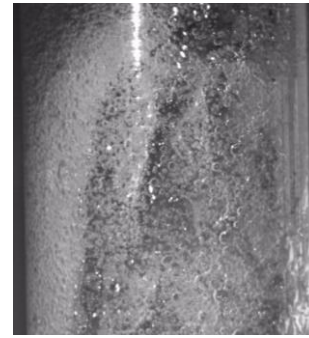
Figure 8: Video image of churn flow for a riser at liquid superficial velocity = 0.142 m/ s and gas superficial velocity = 2.363 m/ s.
