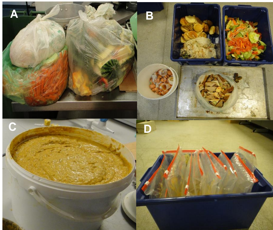
Figure 4.2. Grab sample collection and processing; A) waste sampling from the Refectory, B) sorted samples, C) processed sample, D) blended samples bagged for storage.
