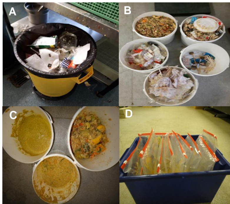
Figure 4.4. Composite sample collection and processing; A) waste sampling from the Refectory, B) samples sorted into categories, C) portions of the processed samples by first mincing followed by blending D) blended samples bagged for storage.
