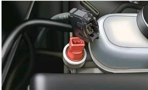
Plate I: Unplugging The Electrical Connector of Brake Pressure Sensor
