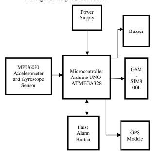
Figure 1: Block Diagram of the System
