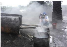
Plate 14: Receiver of Refined Products
