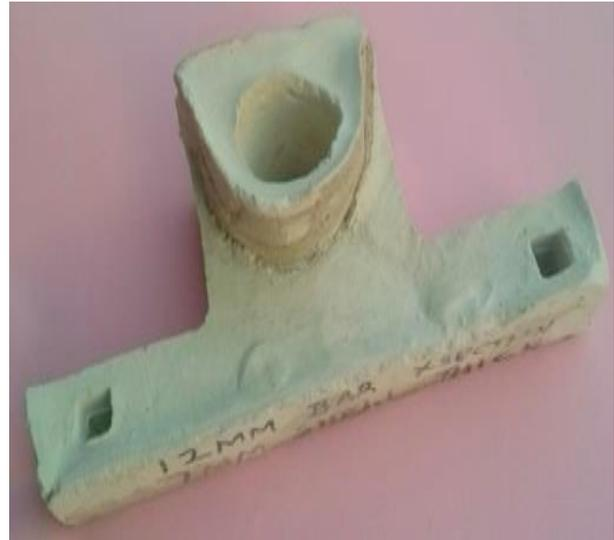
Fig 5: Shell produced after burning of polystyrene and firing
