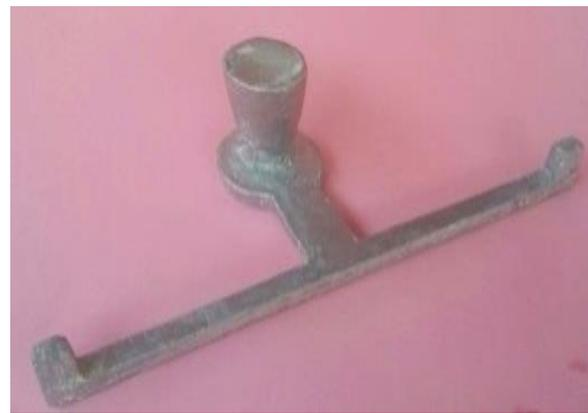
Fig. 6: Bar casting after knockout and cleaning operation
