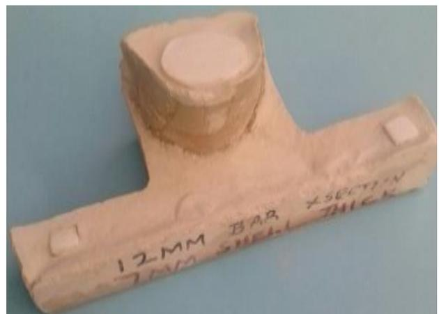
Fig. 4: Bar shell formed and left for drying
