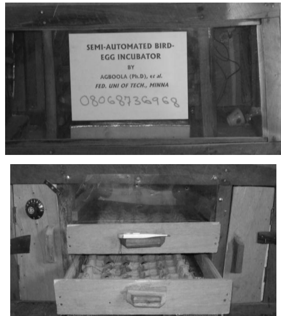
Figure 2: Forced Air (Oil-Lamp) Model of Bird Egg Incubator
