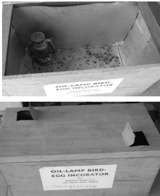
Figure 1: Still Air Model of Bird Egg Incubator
