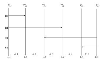
Fig. 4 – Grid diagram of a target based superstructure (TBS) for two hot and two cold streams.
