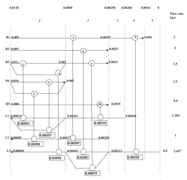
Fig. 10 – The T&SBS network structure of Example 6 featuring nine units with a TAC of \$131,524.
