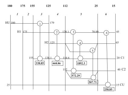
Fig. 6 - Network structure of S&TBS (Types 1 and 2) for Example 2 featuring six units with TAC of \$235,781.
