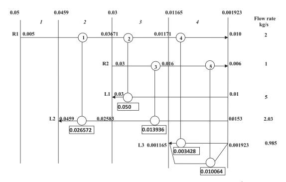
Fig. 11 - The S&TBS network structure of Example 7 featuring five units with a TAC of \$421,147.
