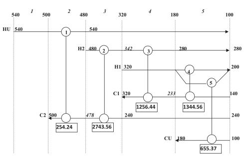
Fig. 5 – The S&TBS (Type 1) network structure for Example 1 featuring five units with a TAC of \$10,786.
