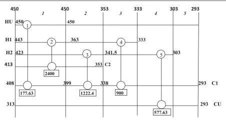
Fig. 7 – T&SBS network structure for Example 3 featuring five units with TAC of 87,611\$/year.
