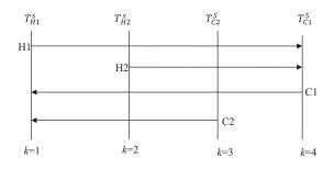
Fig. 1 – Grid representation of the superstructure for two hot and two cold streams.
