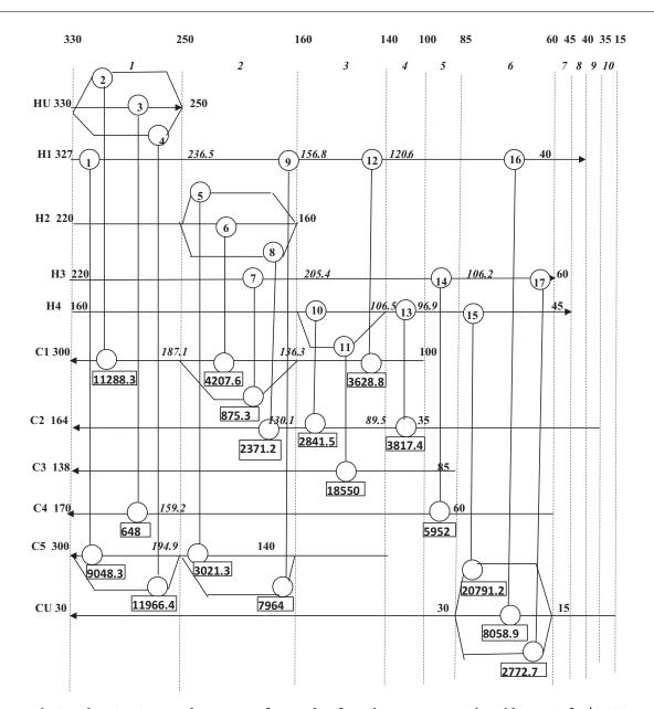
Fig. 9 - The T&SBS network structure of Example 5 featuring seventeen units with a TAC of M\$2.922.
