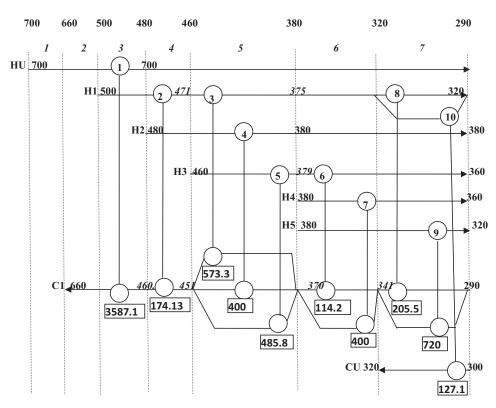
Fig. 8 – The S&TBS (Type 2) network structure for Example 4 featuring ten units with multiple split of the cold stream with a TAC of \$577,602.
