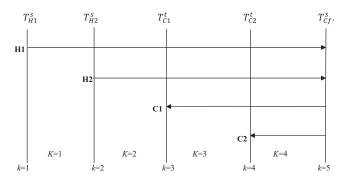
Fig. 2 – Grid diagram of a supply and target based superstructure (S&TBS) for two hot and two cold streams.
