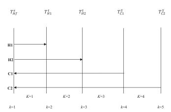
Fig. 3 – Grid diagram of a target and supply based superstructure (T&SBS) for two hot and two cold streams.
