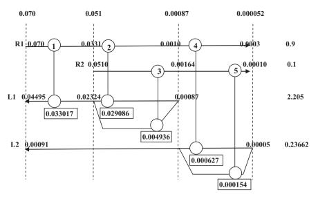
Fig. 13. The SBS superstructure for Example 8 with TAC of 469,968 \$/yr.
