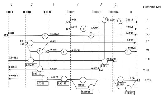
Fig. 11. Network structure for Example 6 of SBS featuring nine units with a split of rich stream and two separate 2 way splits of a lean stream with TAC of \$129,901/yr.
