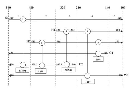
Fig. 5. The SBS network structure with match H1–C1 forbidden featuring five units with a TAC of \$20,019.
