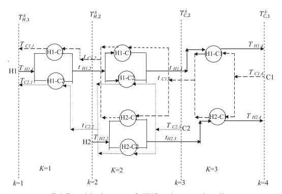
Fig. 2. The supply-based superstructure for HENS for two hot streams and two cold streams.
