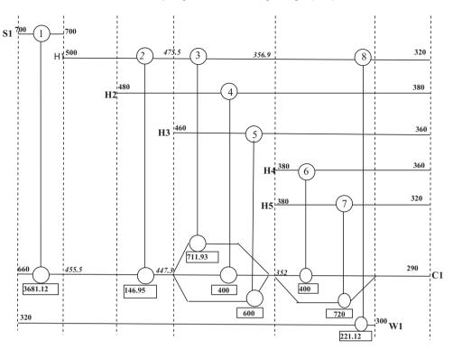
Fig. 8. The network structure for Example 4 of the SBS featuring eight units and one 3 way split and one 2 way split of the cold stream with, a TAC of \$580,023.
