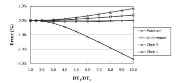
Fig. 3. Comparison of log-mean approximation errors.
