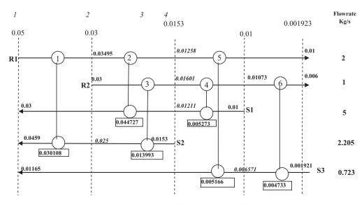
Fig. 12. SBS network for Example 7 featuring six units with a TAC of \$339,579.
