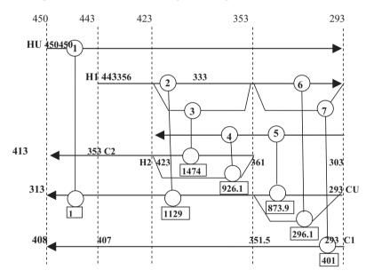
Fig. 7. SBS network structure for Example 3 featuring seven units with TAC of \$90,521/yr.
