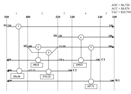
Fig. 4. The SBS network structure featuring five units with a TAC of \$10,794.
