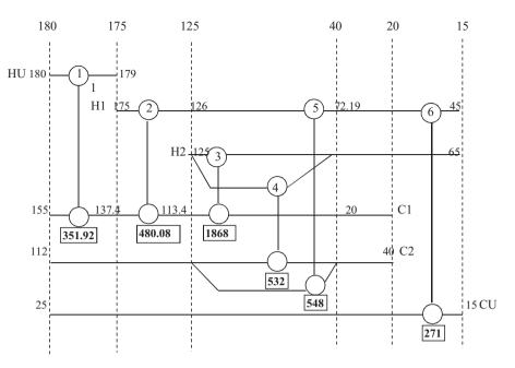
Fig. 6. SBS network structure for Example 2 featuring six units with TAC of \$235,931.
