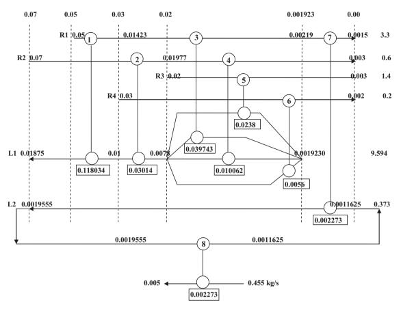
Fig. 14. SBS network structure for Example 9 featuring 8 units with TAC of 693,976 \$/yr.
