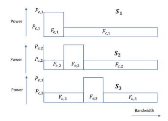
Fig. 3. Standard Downlink Resource allocation for Sectors in S1, S2 and S3
