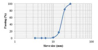
Fig. 2. Particle size distribution curve for coarse aggregates
