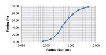
Fig. 1. Particle size distribution curve for fine aggregates
