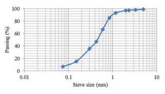
Fig. 3. Particle size distribution curve for RHA
